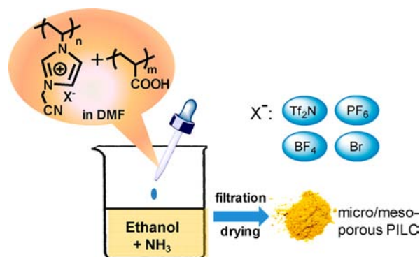
Scheme 1. Synthetic Route to Micro-/Mesoporous PILC Based on PCMVImX PILs and PAA [Tf 2 N = Bis(trifluoromethanesulfonyl)imide]
